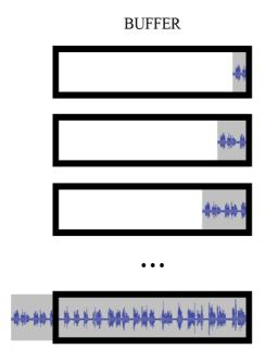
By default, sound is sent to the buffer continuously, just like in an ordinary delay effect. If you flip the *hold* switch, however, the buffer is frozen. The group of amber lights at the lower left front panel provides an overview of the contents of the sound buffer.
